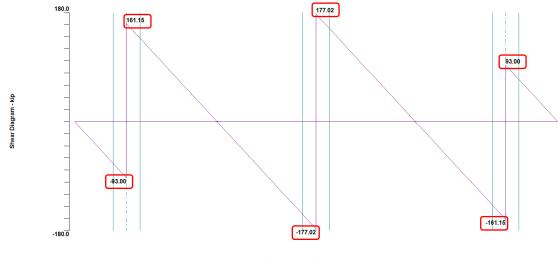
Shear Force Diagram from spSlab
