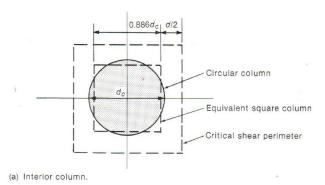
Excerpt from Fig. 13-77 of Wight J.K. Reinforced Concrete, Mechanics and Design, Seventh Edition <sup>[10]</sup> where  $d_c$  equals to the diameter of circular column,  $h_c$ .
