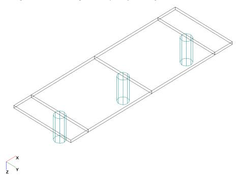
Isometric view of two-way flat plate concrete floor slab supported by circular columns
