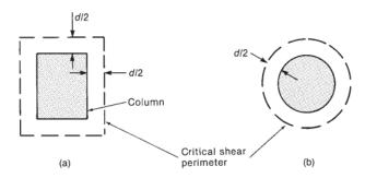
Location of critical shear perimeter – Excerpt from pg. 689 of Reference [10]
